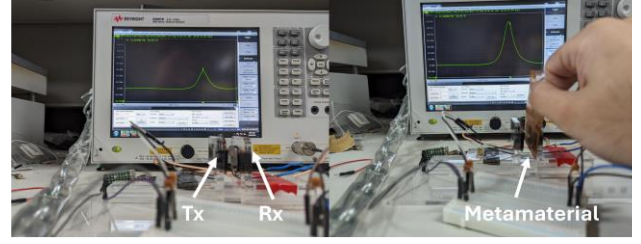
Figure 3: The measured PTE spectrum of Tx and Rx coil antennas with/without metamaterial.
