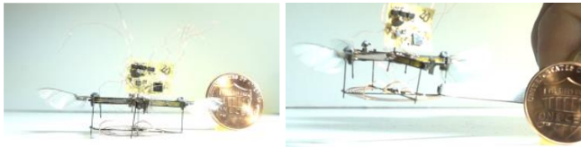
Figure 7: Still-frames of a fully assembled 4-wing robot recording flapping its wings powered wirelessly at up to 1.25 inch distance from Tx coil located underneath the acrylic platform. (right) the robot is gripped by tweezers and lifted above the platform, still receiving enough power to wake the PEU and flap the wings. Here, the 51-AWG wire tether we used for measurement and programming has been cut.
