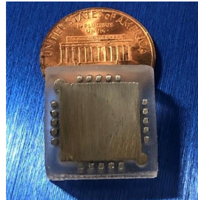
Figure 4: Backside of the final assembled package. The back surface is smooth from the surface finishing and pin isolation
