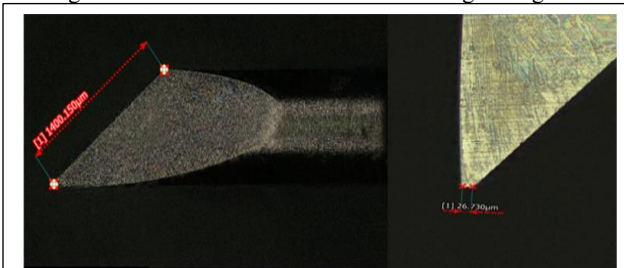
Fig. 2. Laser confocal scanning images of the AutoBlade from the plotter cutter showcasing ellipsoidal curvature on the left and tip dimensions on the right. The blade characterization helps with assessment of cutting features on specific materials.
