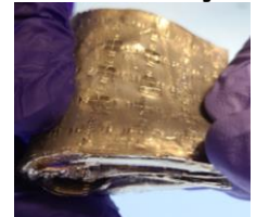
Figure 5. Physical flexibility demonstration of the fabricated metasurface.
