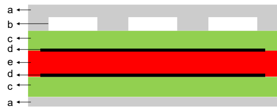
Figure 6: Schematic of the cross-section of the bending actuator. (a) the passivation layer (b) PMMA backbones (c) elastomer layer (d) electrode layer (e) active elastomer layer for actuation.
