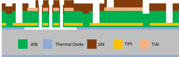
Figure 1. Cross-section of the Piezo-MEMS process flow
