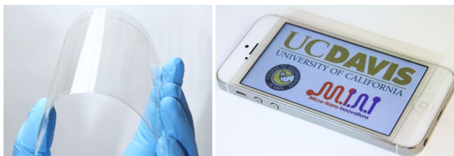
Figure 1: Photographs of the microflotronic film 18 by 10 array with a 5 \times 5 \text{ mm}^2 spatial resolution demonstrating ultra-flexibility and transparency.
