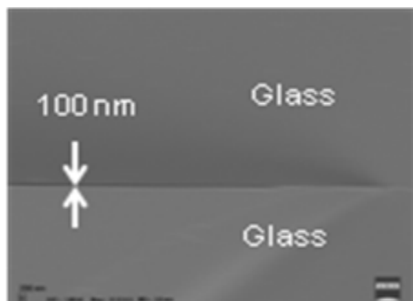
Figure 2: SEM image showing the cross-section of a bonded channel. Part of the slit-like channel with a channel depth of 100 nm is seen.
