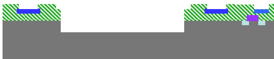
(c) A standard CMOS wafer is fabricated by an independent foundry, and cavities (mask 6) can be etched into the CMOS wafer, if needed for larger clearance under moving MEMS structures.
