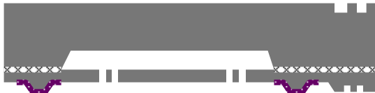
(b) The MEMS wafer is completed by etching the device layer to form standoffs (mask 3) that define the seal ring, the electrical contacts to CMOS, and the vertical gap between the CMOS and MEMS; depositing and patterning a germanium layer (mask 4) over standoffs; and patterning (mask 5) and deep reactive ion etching the device layer to form the mechanical structure.
