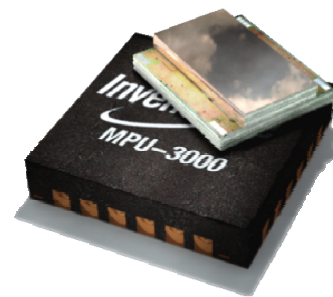
Figure 2: Fully functional, hermetically sealed, 3-axis gyroscope and standard QFN package.
