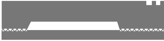
(a) The engineered silicon on insulator (ESOI) wafer is formed starting with a standard silicon handle wafer etched with simple targets for backside alignment (mask 1); followed by oxidation and cavity etch (mask 2). A second wafer is fusion bonded to the handle wafer and subsequently thinned to define the device layer thickness.
