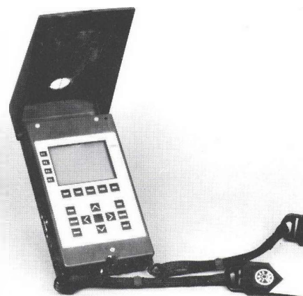
Figure 1. Personal Navigator System Containing Solid-State Compass
